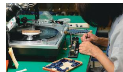
Needle assembly measurement (production line)
